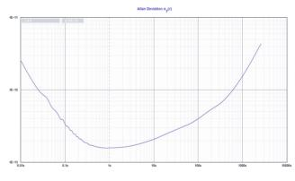
Typical value of the 100ms: 3.5×10<sup>-13</sup> frequency stability: 2.0×10<sup>-13</sup> 10c+ 1.5×10<sup>-12</sup>
